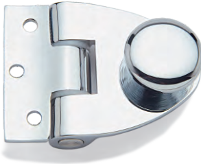
T-2605 DOOR THICKNESS: 6mm to 10mm DOOR WELGHT: 45 Kgs maximum MATERIAL: Brass
