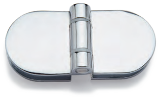
T-2604 DOOR THICKNESS: 6mm to 10mm DOOR WELGHT: 45 Kgs maximum MATERIAL: Brass
